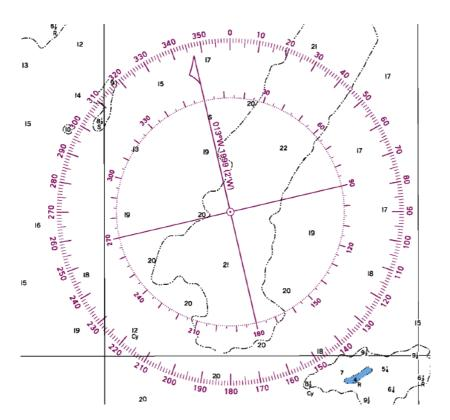
The outer rose is oriented with respect to True North so zero is vertical. The inner rose is oriented with respect to magnetic north (when the chart was issued in 1999). The
